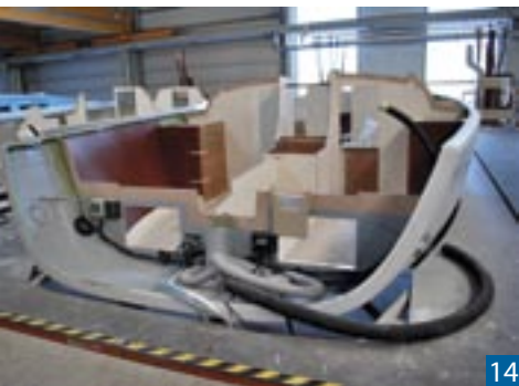
13 Station 1, Line 1 — a hull moulding with strengthening grid already glued in place has its seacocks fitted. 14 A little way up the line, bulkheads, plumbing and cabling are installed. 15 Furniture is fitted. 16 At station 5 on the main assembly line, the deck, complete with fittings, is glued, screwed and laminated to the fully fitted-out hull.
