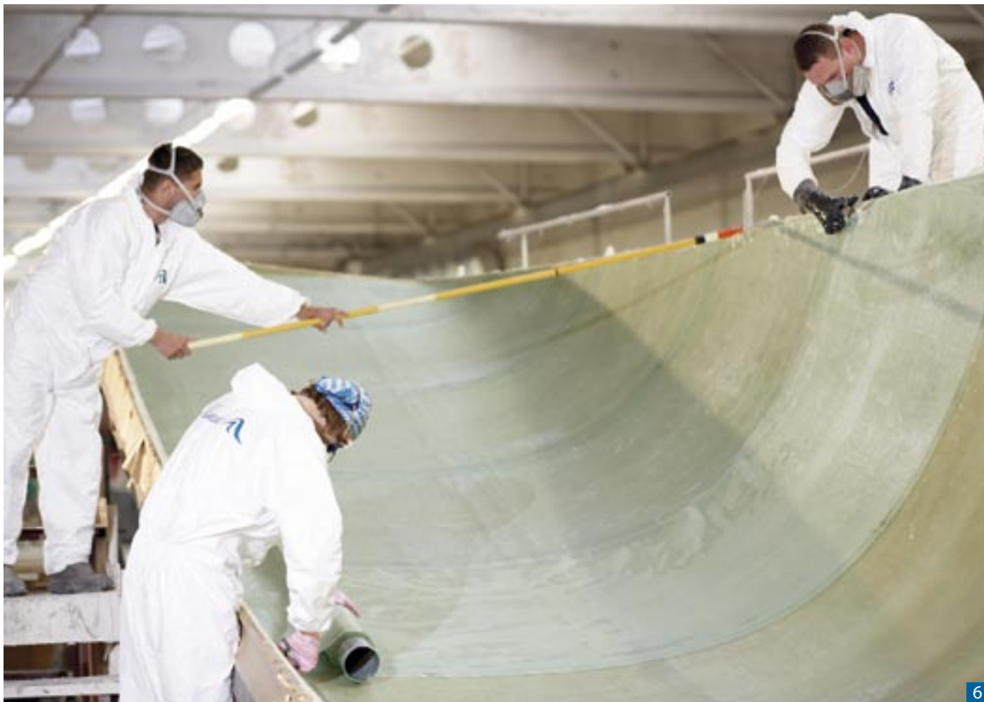
6 Epoxy resin e-glass prepregs are laid in a mould at HanseYachts' lamination plant close to its Greifswald headquarters. A Corecel-core epoxy sandwich laminate is standard on larger Hanse yacht models. 7 An epoxy moulded deck awaits fitting out and finishing at the assembly plant. 8 Hull and deck mouldings in balsa cored polyester are transported by travel hoist across the yard after delivery from Poland.
